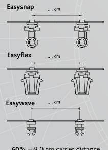
**60%** = 8,0 cm carrier distance **80%** = 6,0 cm carrier distance **100%** = 5,4 cm carrier distance
